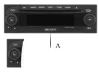
► Slide the button which unlocks the control panel (A) to the right
