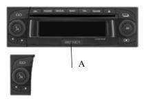
▶ Push the release slide for the control panel (A) to the right.
