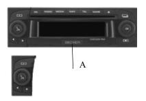
▶ Push the release slide for the control panel (A) to the right.
