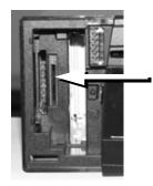
▶ Push the SIM card carefully into the slot.
