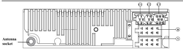
**Warning.** Terminal 30 and Terminal 15 must always be connected separately, otherwise increased power consumption will occur when the unit is switched off. Connection socket A is not the same for all vehicle types. Therefore, always measure voltages before installation.
