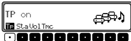
**Switching off:** To switch off TP in the TP menu, press the **TP** multifunction button repeatedly until **TP off** is displayed.
