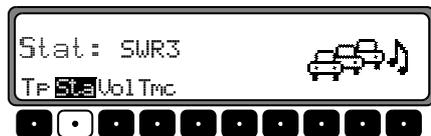
Using the right rotary control
