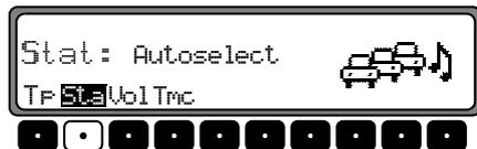
Using the right rotary control
